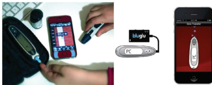
The Bant system includes an iPhone and a LifeScan glucometer with a Bluetooth adapter for automated data transfers to the app.
