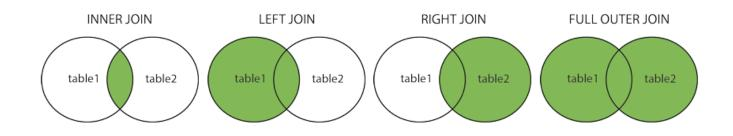
Data in relational databases can be spread across many tables in the database. This is done to enable efficiency at different stages of data maintenance process (writing, querying, updates, etc). Join clauses allow us to merge different columns from different tables based on a join condition.
